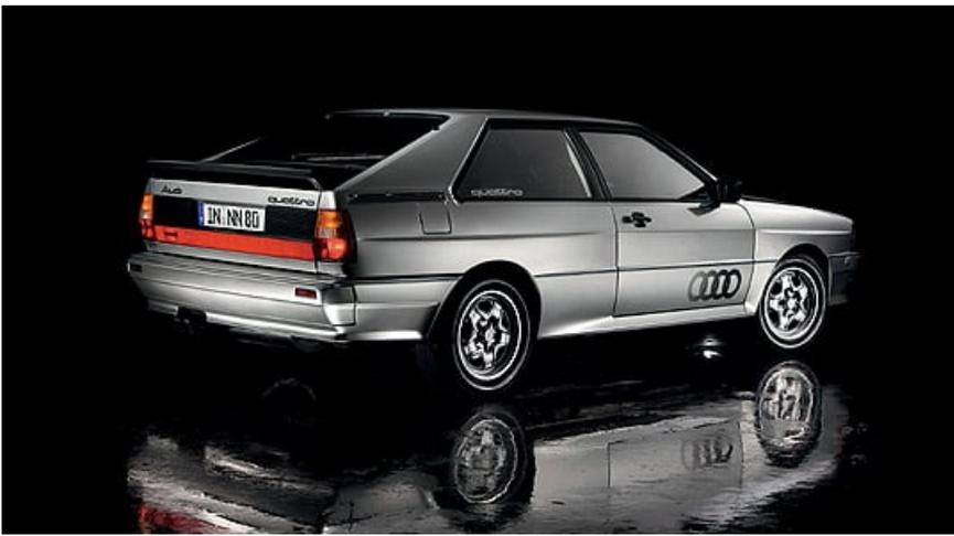
Its five-cylinder engine was something special, too: producing 200bhp from a turbocharged 2144cc, and aided by that all-wheel-drive traction, it could propel the Quattro to 60mph from rest in 6.5 seconds. Impressive mid-range torque enhanced the performance and the feel of the car on the road. The top speed of 138mph might seem modest now, but very few cars could get anywhere near that pace 30 years ago.
