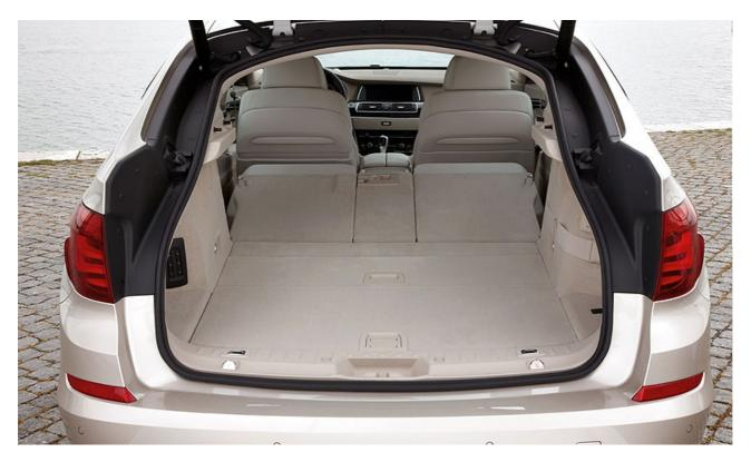
How it works is that a conventional-style boot can be used for small items, while opening the tailgate complete with glass rear window allows almost Touring-like access. The rear seats can be moved 100mm fore or aft to either increase boot space or provide greater legroom for rear seat passengers. With the rear seats in their most forward position, and folded flat, the 5 Series Gran Turismo can swallow surprisingly large objects.
