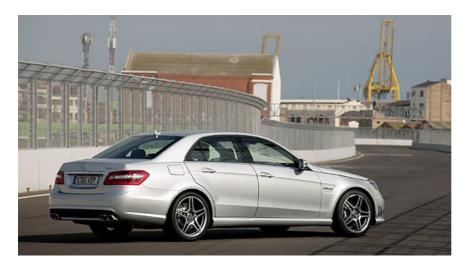
The new E 63 comes equipped with 18in diameter AMG light-alloy wheels shod with 9in 255/40 R 18 (front) and 9.5in 285/35 R 18 (rear) tyres. Externally, the usual array of subtle spoilers and air-vents completes the sporty picture.
