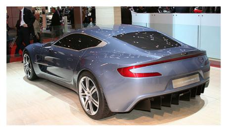
The car is likely to weigh in at 1500kg, will wear unique-to-the-car Pirelli P Zero Corsa tyres (255/35 ZR20 front, 335/30 ZR20 rear), and will transmit its 700+bhp to the road through the rear wheels, via a new six-speed gearbox. The gearbox uses the principles of the company's Sportshift transmission, but is heavily uprated to cope with the extra power and torque. CCM brakes are standard.
