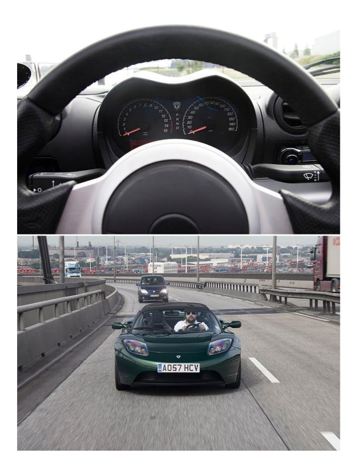
The framework and the carbon body come from Lotus, and were assembled at Hethel. Tesla estimates that the car can travel up to 350km between charges and that a full charge using the High Power Connector (included in the price) takes as little as 3.5 hours, with the car costing around nine euros to 'fill'.
