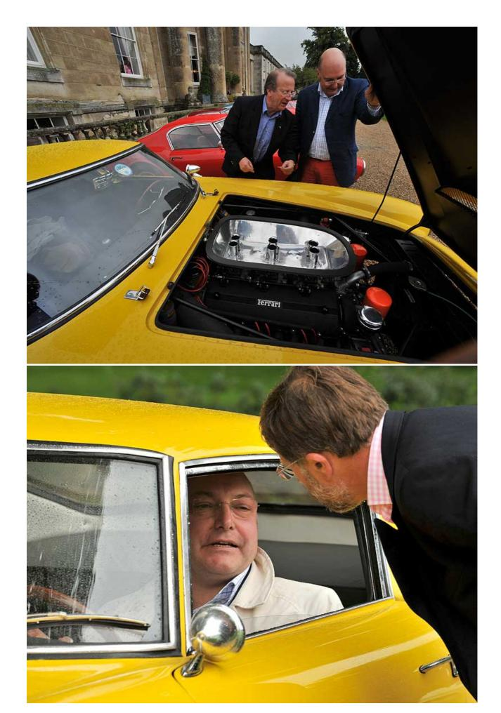
The *Giallo Fly* car you see here is one such. Based on a **1959 250 GT Pininfarina Coupe**, the car was built up by **Giovanni Giordanengo** of Cuneo, south of Turin, in the late 80s. Instead of the familiar 3-litre V12, there's a Tipo 209 engine from a 330 GT, producing around 300bhp from its four litres and mated to a four-speed Ferrari transmission.
