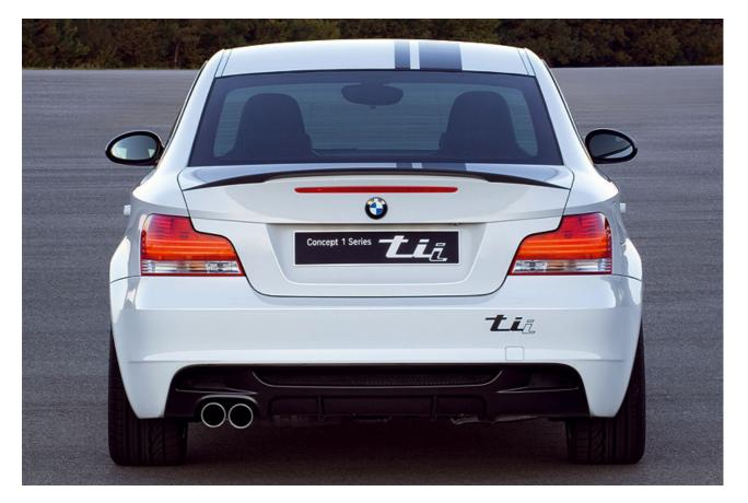
The optimised aerodynamics include reshaped bumpers and sills, plus special gurney flaps generating additional downforce on the rear axle. The principles of 'lightweight engineering' ensure the widespread use of carbonfibre components – such as bonnet, mirror caps, air-scoops and so on – resulting in a significant weight reduction against the series production cars.
