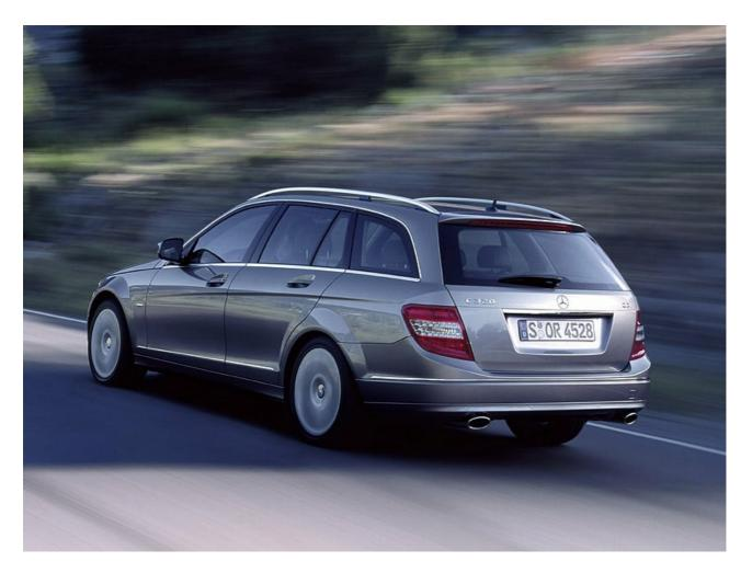
If you take the normal features of the new C as the saloon, the news on the estate version is that it is more capacious than before with a load area that now varies between 485 and 1500 litres (VDA measuring method), depending on the position of the 1/3 : 2/3 split-folding rear seat.
