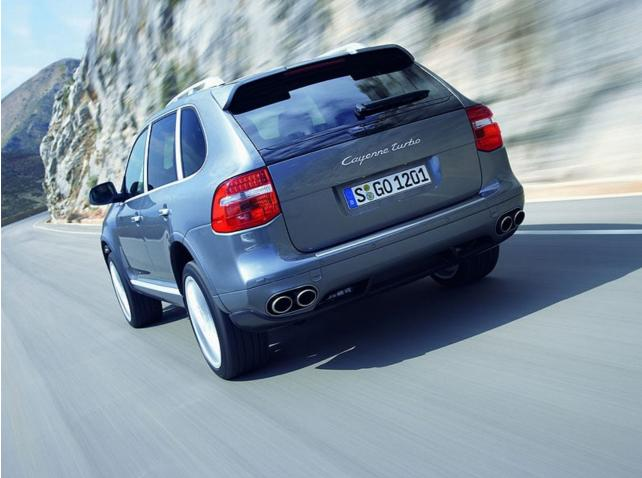
The Cayenne Turbo is fitted with Porsche Active Suspension Management (PASM), with air suspension as standard. This variant can now be augmented with the new Porsche Dynamic Chassis Control (PDCC) roll stabilizer system. This constant roll control, also available for the Cayenne and Cayenne S, limits vehicle roll in corners and counterbalances it completely in most driving situations.
