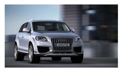
Trading on their overwhelming succes in sports car racing this year with the Le Mans-winning R10s, Audi has announced the world's first production V12 diesel. The six-litre V12 will makes its debut in the Audi Q7. It produces a colossal 500 PS and 1,000 Nm of torque.
