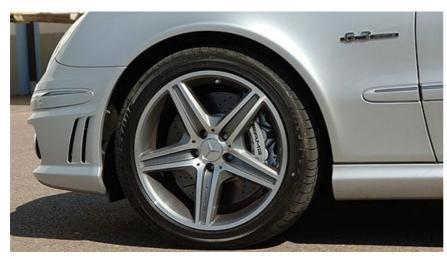
And once you've wound the big car up to terminal velocity you don't need to worry about the braking. Slowing from speeds above 180 km/h is of the order of racing cars from just a few years ago. Eight-piston light alloy callipers at the front working in co-ordination with the very latest DaimlerChrysler electronics ensure the finest stopping power around. When the car detects an 'emergency' level of braking it will activate the hazard warning lights too.
