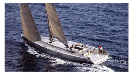
Roma has been designed as if an America's Cup contender, patient work in the distribution of the fibres and the precise respect of the weights has allowed the boatyard to even improve on the theoretic values. The hull, deck and structure have been built with the same materials, methods and skills utilised to build the Transpac 52', the latest racing boat launched by the shipyard.
