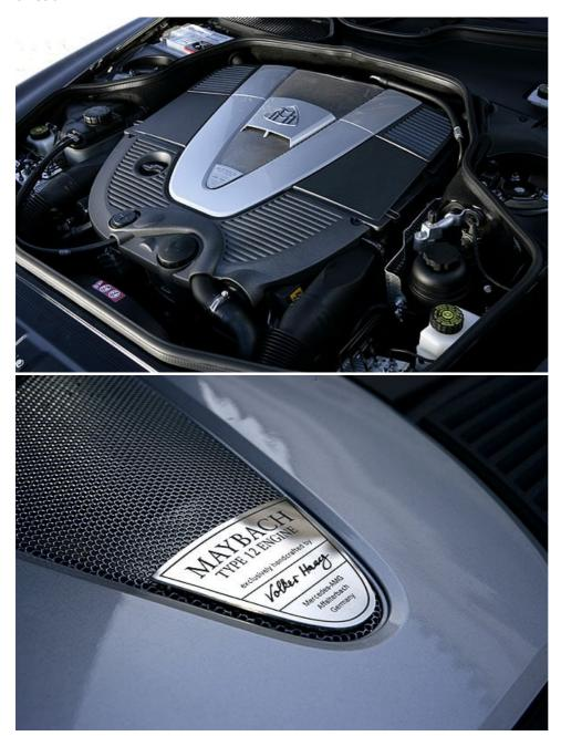
But the world is not entirely composed of curves, and after the final corner the full power of the engine can be released. As soon as the tacho reads 2,500 rpm it's all systems go. The hand-built (by AMG, with twin water-cooled turbos) V12 has a capacity of 6.0 litres and produces 615 HP to give the car an electronically-limited top speed of 275 km/h (171 mph), the fastest for a series-production German saloon. But the hard,
