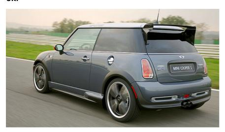
The MINI Cooper S with JCW GP Kit will be a two-seater in exclusive colours, and extra safety and interior options will come as standard. The reduction in weight over the standard MINI Cooper S has been achieved by modifications to the chassis and engineering tweaks. The longitudinal control arms on the rear axle are now made of aluminium, and the omission of the sound-deadening material and the rear seats have made further weight reductions.
