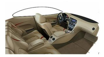
More innovations internally include the re-arrangement of switchgear and instruments to utilise the space gained by the (now common, due to the F1 paddle-actuated gearbox)) deletion of a gear lever in the central console, thus freeing up space for the light switches and electronic handbrake. The rest of the instrumentation is standard 612 Scaglietti, however the dashboard is new and includes a AVIC - X1R Pioneer satellite navigator, fitted right in the centre.
