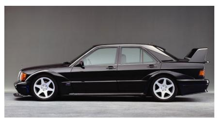
The EVO II stood out for its bodywork modifications designed to reduce drag still further and to raise downforce at the front and rear axles. Particularly distinctive and eye-catching features were the large rear airfoil and the wheelarch flares.
