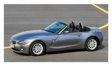
BMW is pleased to announce the arrival of the Z4 2.0i Roadster, a new entry-level model for the two-seater, open top sports car. Powered by a 150bhp engine, the new car is the first Z4 to be fitted with the lightweight four-cylinder powerplant built at Hams Hall, Warwickshire, UK. The 1,995cc unit propels the Z4 from zero to 62mph in 8.2 seconds before going on to a top speed of 136mph. Torque is 200Nm at 3,600rpm.
