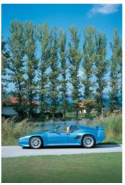
The Pantera chassis has always been a steel monocoque construction with a mid-engined layout. The first models from 1970 produced 310bhp and weighed 1455kg (213bhp/tonne). In 1973 came the GTS still with the 5763cc Ford V8. Over the years, the factory offered three axle ratios (std 4.22:1, 4.02:1 and the so-called 175mph Le Mans axle with 3.77:1) and performance varied accordingly.
