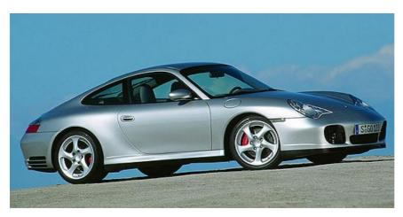
Measuring 350 millimetres or 13.78" in diameter, these cross-drilled, inner-vented composite ceramic brake discs weigh approximately 50 per cent less than metal discs and reduce unsprung masses on the Carrera S by 14 kilos or 34.4 lb. In conjunction with the brake pads also quite different in design and material, the ceramic brake discs immediately build up a high and, in particular, consistent level of friction during application.
