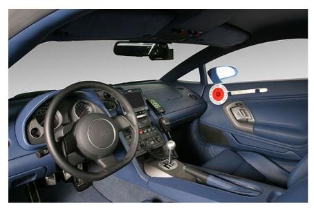
The car also carries full Police radio and communications equipment such as a satellite navigation system (via GSM telephone), VHF radio, and two special technical systems developed for the Italian Police; "Provida" which connects the car to the national criminal record database and "Elsag", an automatic numberplate recognition system.
