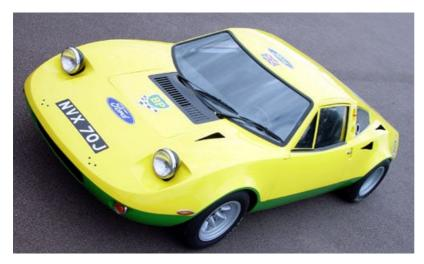
Restoration began early in 2002 at Sporting and Historic Car Engineers' premises in Poundon, Oxfordshire. Fortunately, most of the competition components including the ventilated disc brakes with four-pot calipers, driving lights, instruments and Minilite wheels were kept with the car. Standard Ford parts were used to replace other components on the vehicle.
