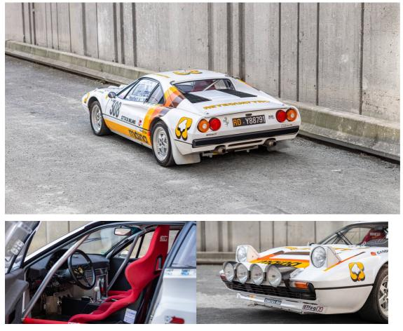
Having made its debut at the 1975 Paris Motor Show, the Ferrari 308 GTB was the model selected for a rally makeover. Unlike Ferrari's V12 berlinettas, the 308 GTB featured a transverse V8 mounted behind the driver, improving its weight distribution and cornering ability. Meanwhile, its tubular frame construction meant that it was relatively simple to replace the production body with lightweight fibreglass panels.
