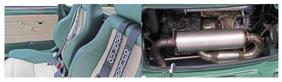
The Meanie is mid-engined, rocketed along by an in-line four-cylinder engine with direct injection and a turbocharger from Volkswagen, producing an impressive 189 horsepower. The chassis consists of a specially developed tubular frame made of chrome-molybdenum steel, while the bodywork remains incredibly modest, leaving only the sharpest of eyes to spot what lurks beneath this mighty Meanie.
