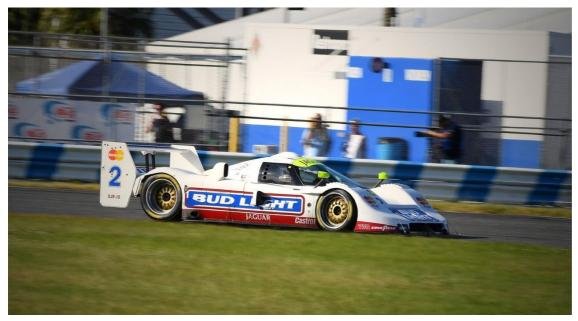
Dubbed the XJR-16, this cutting-edge big cat was powered by a 90-degree twin turbocharged V6 engine sending between 750 to 900 hp to the rear wheels only via a TWR fivespeed manual gearbox. Not only did it look the part and have enough shove to back up its visual bite, but the - weighed in at a scant 950 kg, giving it quite the impressive power-to-weight ratio.
