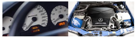
Despite the wallflower appearance, the C43 packs a punch, thanks to its bulletproof 24-valve 4.3-litre V8 pushing out 302 horsepower via a 5-speed automatic. While by no means a drag strip demon, the C43's quoted 0-60 mph time of 5.9 seconds and 155 mph top speed make it a brisk saloon by modern standards, and certainly far swifter than the 'Sport' bodykit — shared with lesser C-Class models — would suggest.
