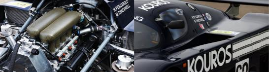
The new C8 car represented a major technological leap forward, thanks to its aluminium monocoque chassis which was fitted with a Kevlar-reinforced fibreglass body designed by Peter Faul. While the C7 remained naturally aspirated, the C8 was given a monstrous power upgrade in the form of two turbochargers, good for almost 650 horsepower, which could be wound up to an incredible 800 horsepower for those last-dash qualifying runs.
