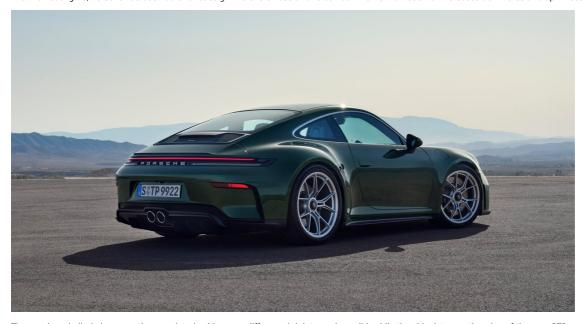
The rear has similarly been gently re-sculpted, with a new diffuser, air inlets, and rear lid, while the sideplates on the wing of the new GT3 are more angular. The wingless Touring model gets a new special badge on the rear lid grille, while its extendable rear spoiler now features a Gurney flap for a hint of added aggression. Another first on the Touring model is the option to add rear seats, finally cementing it as arguably the ultimate 911 for daily duties.
