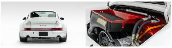
Finally, the engine was similarly overhauled, gaining 61 horsepower over the standard car thanks to more aggressive cams, larger fuel injectors, and a more efficient KKK turbocharger, resulting in a total output of 381 horsepower at 6,000 rpm. So, if you want to experience the 911 Turbo in one of its most raw and brutal forms, step this way!
