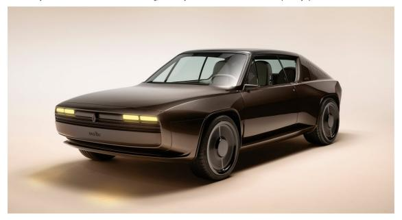
Using the 'same but different' mentality, the original 17 had a plucky engine that had enough performance in the streets and on the open road, which has now been swapped for an all-electric 270 hp powertrain, nestled into the rear. The carbon fibre chassis features flush lines, designed to keep the weight down to just 1.4 tonnes and retain the car's sleek stature.
