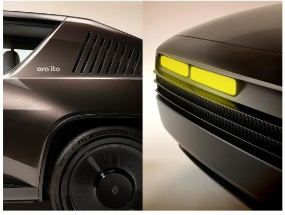
Now, they have done it again with the freshly launched R17 electric restomod x Ora Ïto, a sculptural retake on the original model launched in 1971, and we are a little bit in love. Based on the monocoque structure of the original, the R17 electric has the same cabin, doors, windows, glazing, seals and underbody, all of which given a modern touch, with its body now 17cm wider to enhance roadholding, with boxy wheels arches for an almost Group B rally specification look.
