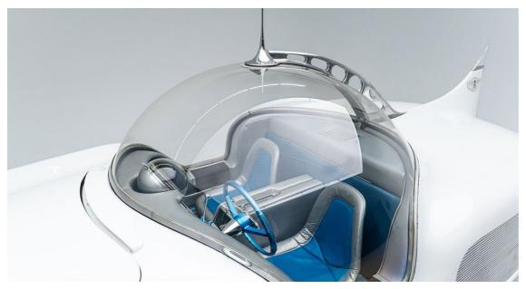
He specified a shaped, jet-like Plexiglas canopy that could be raised and lowered by an electric motor connected to an aluminium arm and which, when opened, allowed driver and passenger to climb in and out via stepped sides. As well as providing all-round vision, the canopy made for a light and open feel and, with the car's air conditioning on full blast, probably gave the impression of travelling in a convertible.
