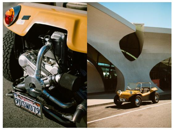
Through a joint venture with Bespoke Engineering, Meyers Manx has created a modified version of an aircraft engine to power its vehicles, a charming byproduct of conversations among car enthusiasts with a penchant for aviation history.
