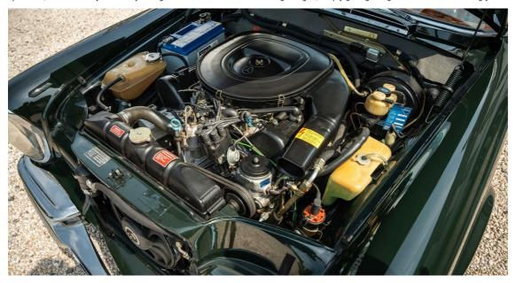
This 1972 example has one final ace up its sleeve, or rather under its bonnet. This emerald drop-top has been lovingly converted to house a powerful 8-cylinder engine, sourced from a W126 500SE from 1981. Additionally, the rear axle from a 6.3 with a differential lock has been installed to ensure optimal driving performance. With just over 231 horsepower on tap, it's likely that new heart transplant has certainly given this W111 even more road presence, if that's even possible!
