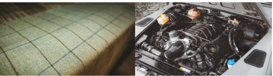
Despite looking similar to the original Land Rover, this modern interpretation certainly packs more of a punch. The Islay Edition is powered by a 405hp 5.0-litre V8 petrol engine, mated to an eight-speed ZF automatic transmission. Each one is comprehensively restored, re-engineered and upgraded, utilising donor vehicles from 2012-2016.
