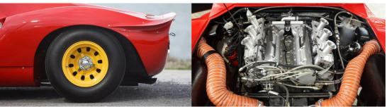
But Drogo's aerodynamic coachwork – made from stressed alloy panels and glass fibre attached to a tubular frame – combined with the most highly tuned, fuel injected, 217 horsepower version of the celebrated 'Dino' V6 engine made the 206S a force to be reckoned with.
