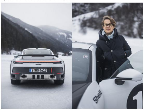
With the reprogrammed four-wheel drive system (locking differential is standard, but the system generally favours the rear wheels), rear axle-steering, active PDCC anti-roll stabilization and a 'Rallye Launch Control Mode' which allows a bigger wheel slip on loose surfaces, it's also no slouch when it comes to devouring an ice track with a few jumps on it. All that on standard winter tyres.
