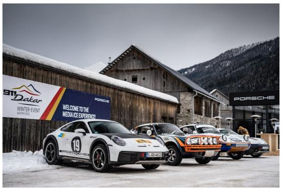
The whole setup is incredibly clever. This beefed-up car sits 50 mm higher off the ground than a regular Carrera, but can raise itself an additional 30 mm if the terrain requires more clearance. Speaking of which, thanks to its short wheel base, the Dakar's ramp angles for approach and departure rival those of conventional SUVs. And its brake-over angle is even better. This allows it to surf dunes like it's Kelly Slater.
