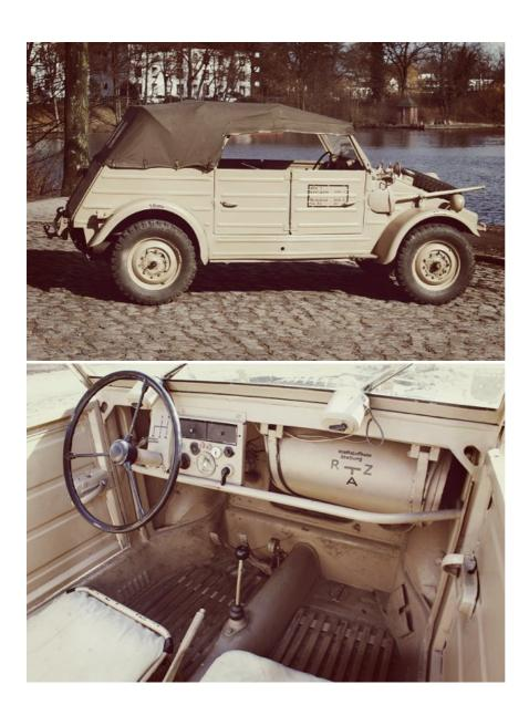
Resembling a bathtub on wheels, it's little wonder the Porsche-designed Type 82 was given the nickname 'Kübelwagen' – directly translated as 'tub-truck'. The Beetle-derived mechanicals proved solid during their service in WWII but, should you get stuck, you could always liberate your mount the old-fashioned way: using the accompanying shovel.
