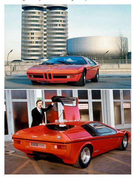
A series of summits in the early 1970s had put a greater focus on safety in the automotive industry, and BMW used the Turbo as a guinea pig for several technologies. It featured an integrated rollcage, a collapsible steering column and a radar-based brake distance warning system. Also, the cockpit was orientated towards the driver to prevent him having to stretch to reach the controls (a now-famous BMW characteristic), while deformable structures were used front and rear to absorb impact.
