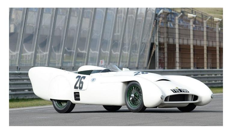
Just a year or so on from the boxy Mk VI and the work of De Havilland Aircraft aerodynamicist Frank Costin is becoming evident. The super-lightweight (the completed chassis/body unit for this model weighed less than a set of five wheels and tyres...) Mk VIIIs are rare – and attractive in the all-white finish of the famous ex-Tip Cunane car you see here.
